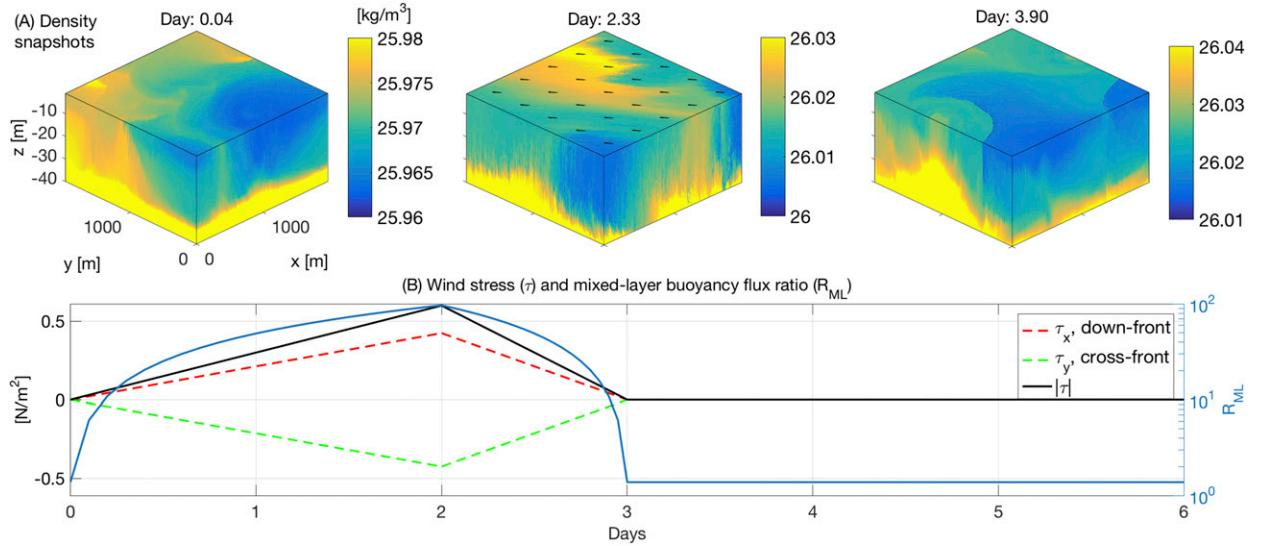
FIG. 1. (a) Snapshots of density and (b) time series of wind stress magnitude (black) and vector components (dashed red and green) as well as the mixed layer buoyancy flux ratio  $R_{ML}$  [see (1)]. Black vectors in the snapshot at day 2.33 indicate the direction of the wind during the storm.
