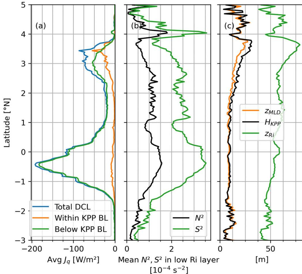
FIG. 12. Meridional profiles of quantities averaged within the low Ri layer at 110°W during the duration of the TIW. (a)  $J_q$  averaged over time and depth. (b) Mean  $N^2, S^2$  within the low Ri layer. The mean is taken over time and depth axes. (c) Time-mean  $z_{MLD}, H_{KPP}$ , and  $z_{Ri}$  over the period when the deep cycle is active.
