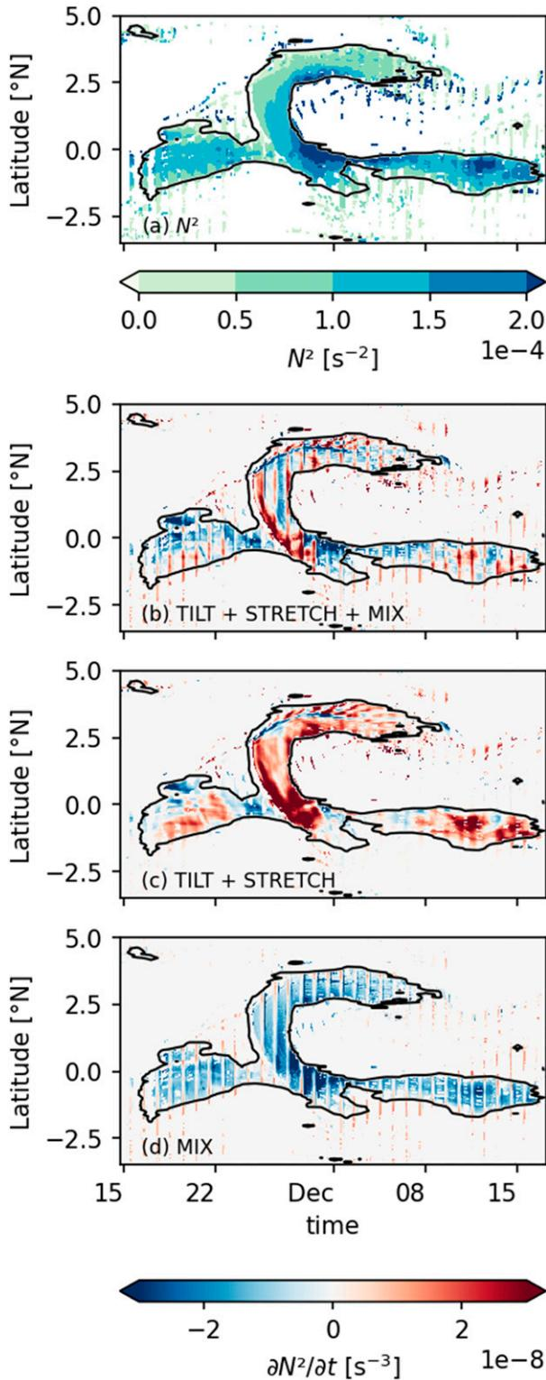
FIG. 10. Time-latitude plots of (a)  $N^2$ , and (b)–(d) the stretching, tilting, and mixing terms that contribute to  $DN^2/Dt$  [from Eq. (9)] within the low Ri layer. The low Ri layer thickness is larger than 30 m within the black contour.
